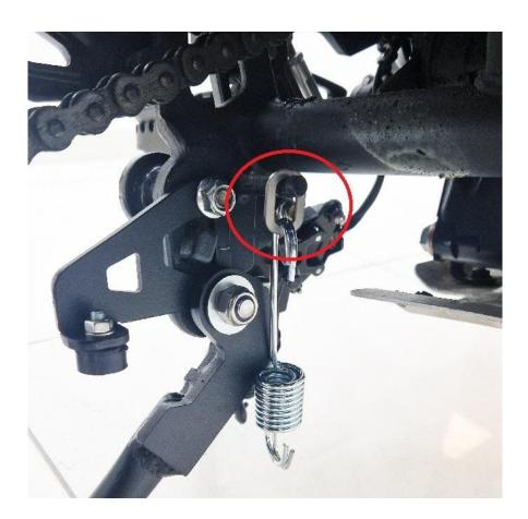
**Step 5:** Install part J and attach the spring side S1 on part J and side S2 on the centerstand hook.
